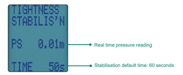
When complete press **ENTER** to start tightness test:
