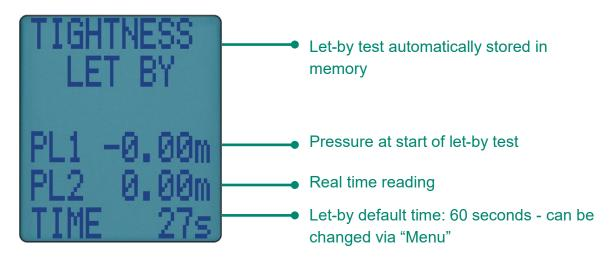
If let-by test fails rotate dial to another position to stop test.
